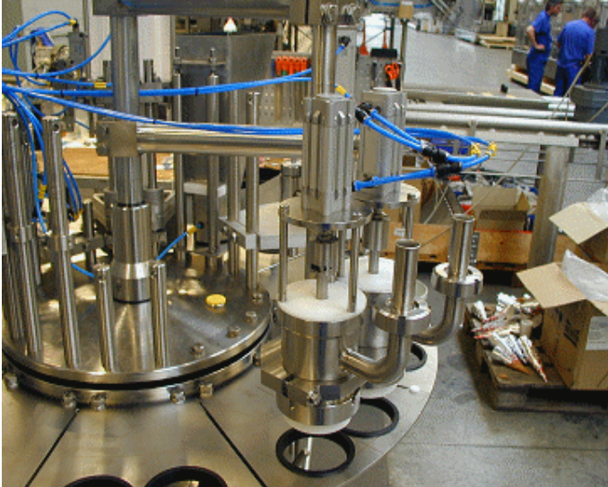
Specially designed "Spaghetti" ice cream filler
